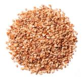
**Granules** through 8/64" over 4/64" RHS\* (through 3.2 mm over 1.6 mm)
